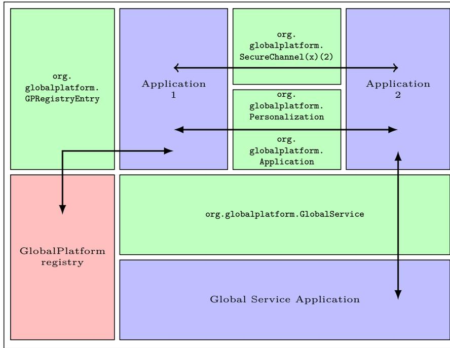
**Fig. 4.** Depiction of an accurate use of the GlobalPlatform API at runtime. Applications are represented in blue color, interfacing tools are in green, while the GlobalPlatform registry, as a database component, is red.
