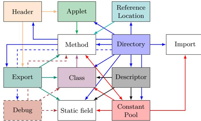
**Fig. 7.** CAP components dependencies. A component pointed is referenced by the component at the other extremity of the arrow. Only the Method component has a double dependency on Constant Pool component. A token in the Method component refers to an entry in the Constant Pool component which may refer to a method in the Method component. Dashed arrows link dependencies to or from debug component.
